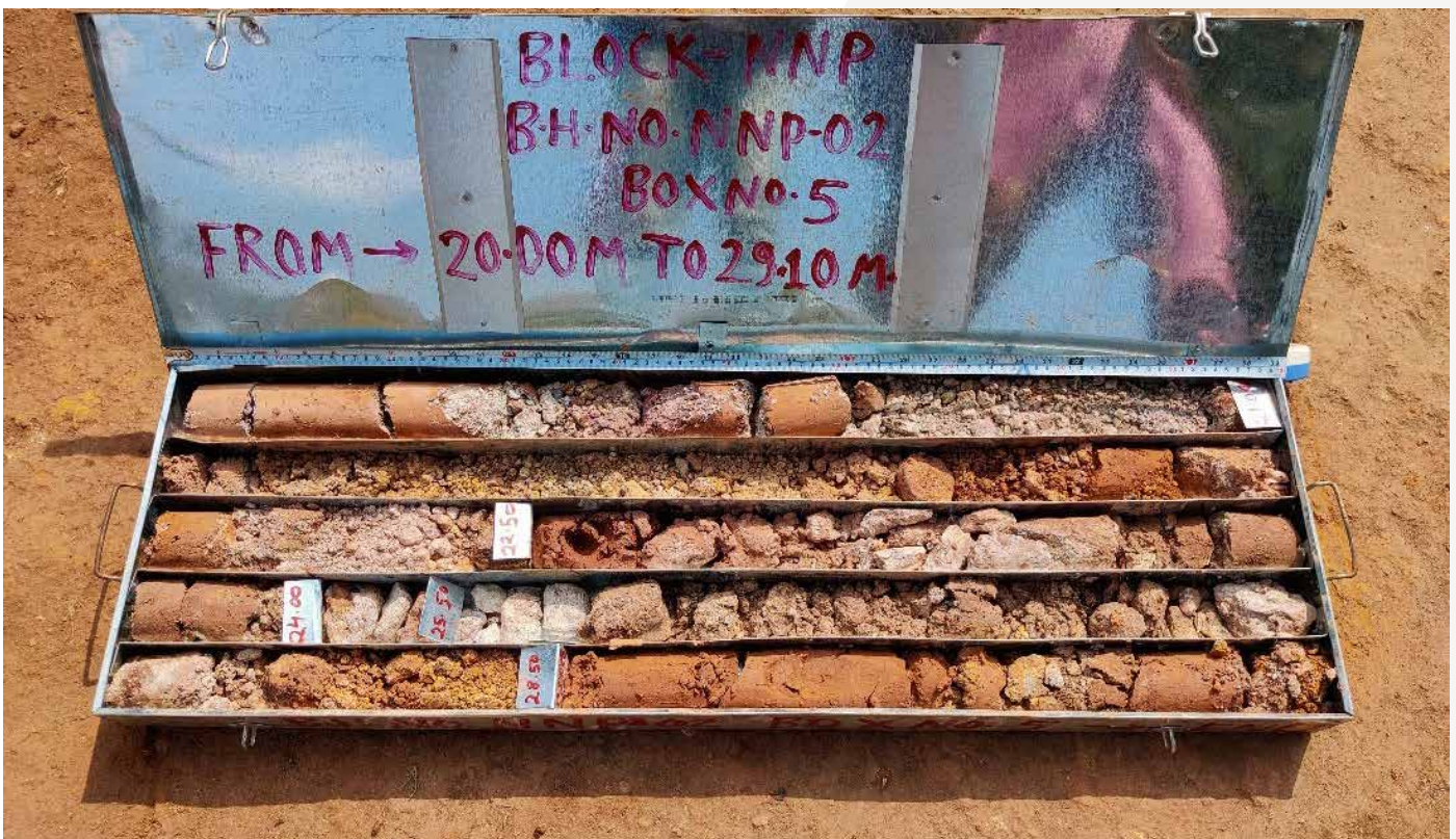
Core samples of Nunapaimali Bauxite Block, Rayagada District, Odisha
